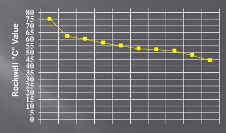
The picture on the left shows .0002" compound (white) layer supported by a nitrogen rich (dark) diffusion zone. The graph on the right exhibits a typical microhardness traverse on H-13 with DYNA-BLUE 6B cycle. The first value is 75HRC at .0002" with each descending value equal to .001".
