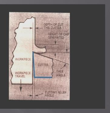
DOES NOT REQUIRE RE-DYNA-BLUE® AFTER FACE SHARPENING AS DYNA-BLUE® IS STILL ON THE LEADING EDGE. PVD COATINGS USUALLY REQUIRE RE-COATING AFTER EACH SHARPENING WHICH INCREASES TOOL COST.
