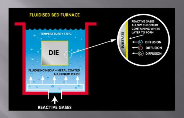
The fluidized bed furnace is capable of maintaining temperatures of +/-2 °F. Inert, atmospheres are introduced through the bottom of the furnace while the furnace shell/retort is electrically heated. As the retort heats, the inert gas scrubs the heat off the walls transferring heat directly to the dies, much like that of boiling water. When the furnace reaches the desired set point, the DYNA-BLUE ® reactive gases can be introduced, providing excellent case depth uniformity.
